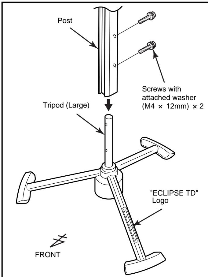
( 2 ) Assemble post and tripod (large)
